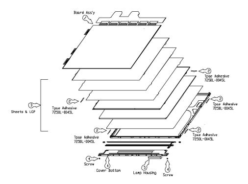
Figure 4-65 Replacing LG. LG. Philips fluorescent lamp (WXGA) (4)
